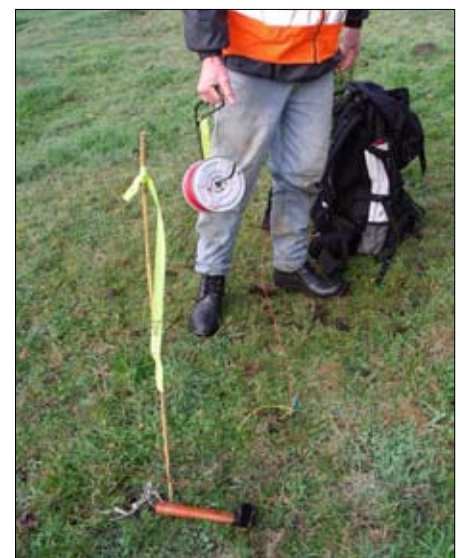
current is injected from each station (yellow and green) - the current travels through the subsurface, and is measured at each receiving electrode (green) inset: example of 3-D data view obtained
