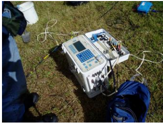
Resistivity receiver in operation in the field
